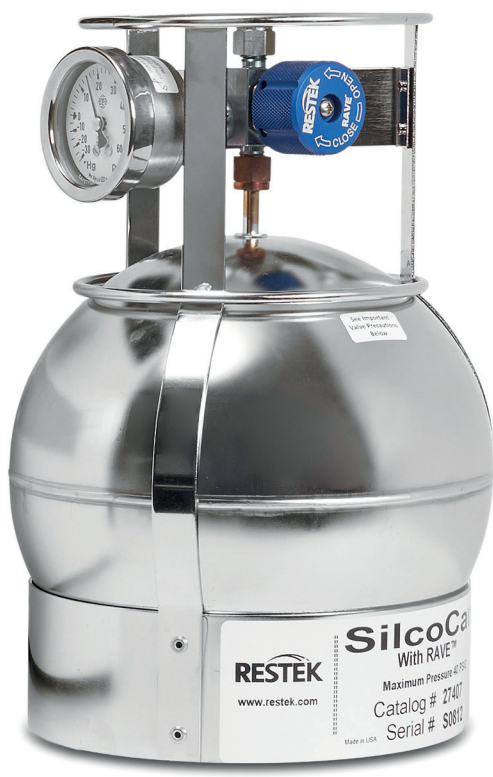
Figure 1: Silicon ceramic lined canister for VFC analysis
