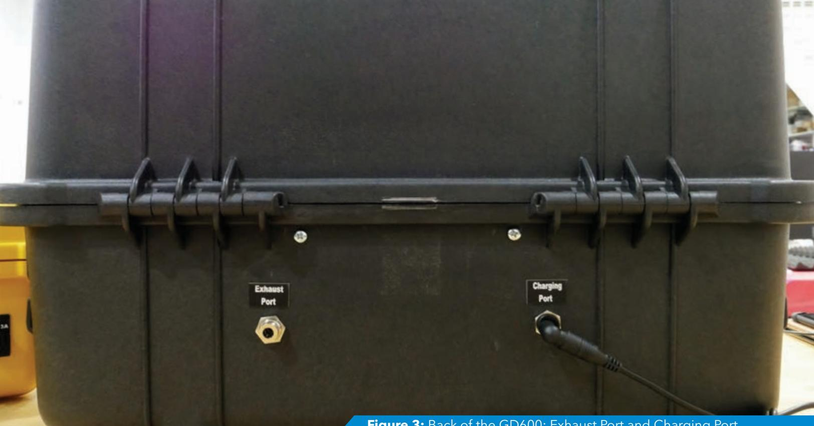
**Figure 3:** Back of the GD600; Exhaust Port and Charging Port
