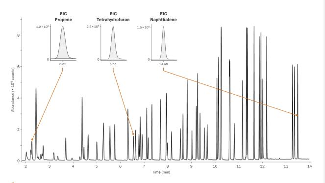
Routine analysis of air toxics by TD–GC–MS with hydrogen carrier gas reduces analytical cycle time to <15 minutes whilst maintaining method performance, method compliance and critical separations across the volatility range.
