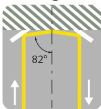
Thanks to the geometry of the Agilent Grazing Angle accessory, it is possible to measure on curved surfaces such as pipes without the aid of other accessories.
