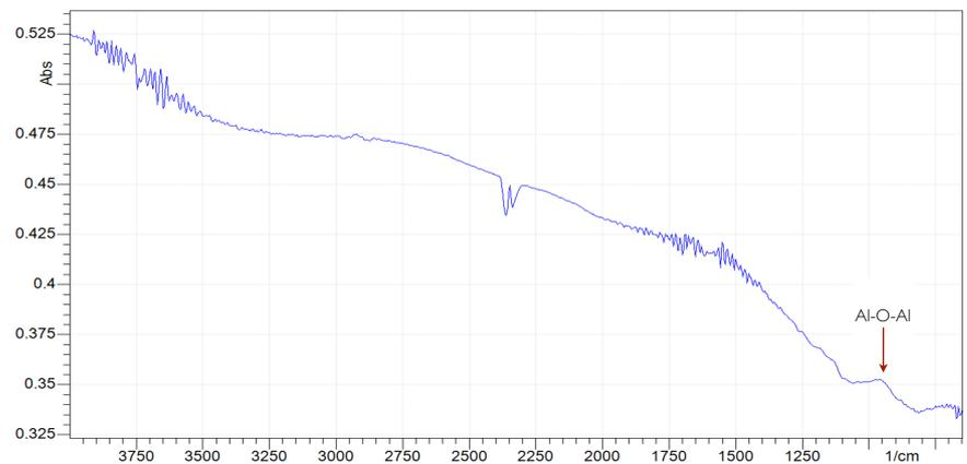
Figure 2 - FTIR Grazing Angle spectrum of an aluminum tube
