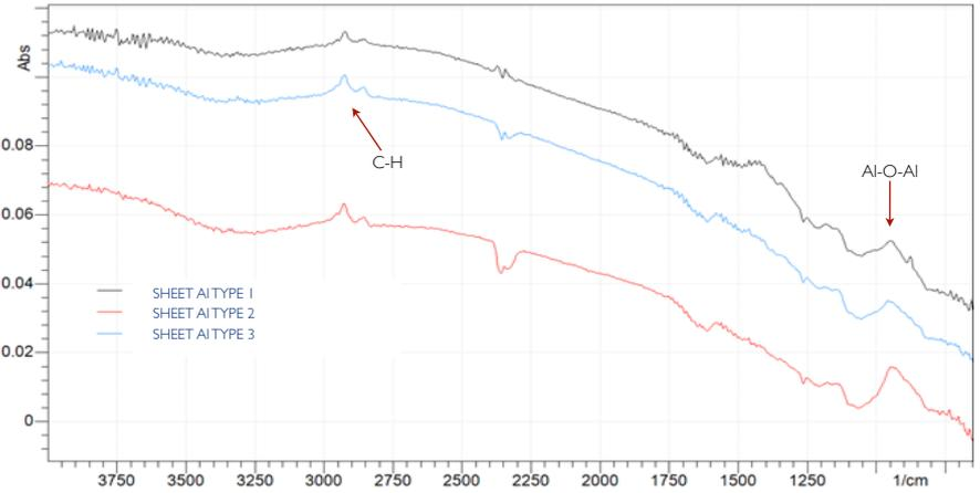
Figure 1 - FTIR Grazing Angle spectra of aluminum sheets
