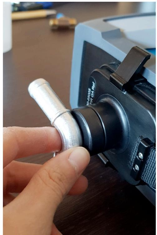
The quantitative data obtained are extrapolated using a PLS1 chemometric method that correlates the intensity of the oxide band with the temperature to which an aluminum sample should be subjected to obtain the corresponding oxide layer. The data obtained is therefore a temperature data that allows to know the oxidation state of the surface of the material.
