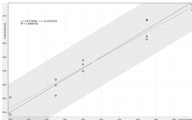
Figure 3 - Chemometric method PLS1 correlating Absorbance vs Temperature
