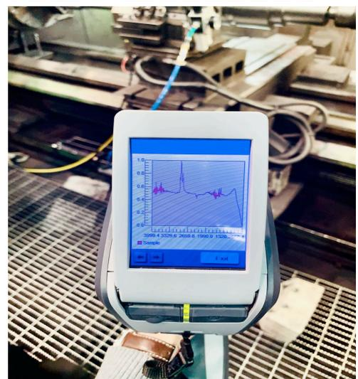
Thanks to the geometry of the Agilent External reflectance accessory, it is possible to measure on curved surfaces without the aid of other accessories.
