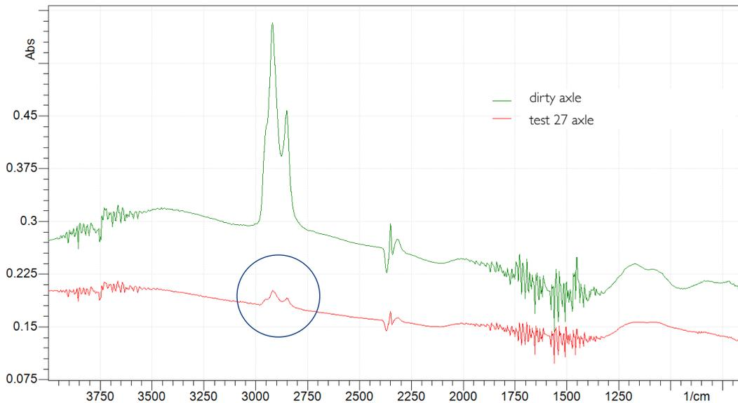
Figure 6 - Comparison of the cleanliness level of a heavily soiled axle. It is possible to notice traces of organic contaminants also following the cleaning process (detail circled in blue) which leads to the piece being rejected as it is not suitable for painting.
