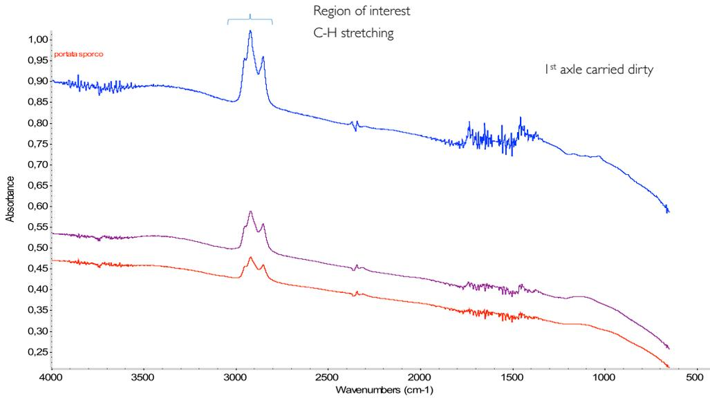
Figure 4 - Specular reflectance analysis of a dirty axle before treatment. The analysis was performed in three points.
