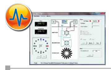
• The **SRA IST software** allows to edit the storage sequence, save the methods, view the status of the instrument and automatically manage the start of the GC analyses.
