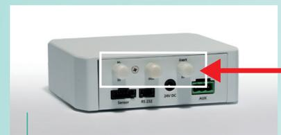
rear panel of external sensor box with module for carrier gas switching
