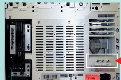
7890 GC rear panel with module for carrier gas switching (see arrow)
