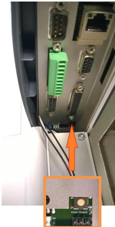
The reset button can be accessed on the main board (see pictures above). To restore the factory default IP address, follow this procedure:
