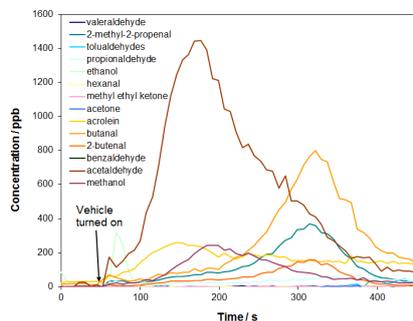
Figure 2: Real-time concentrations of selected hydrocarbons and nitrogen-containing compounds in the exhaust gases emitted by (a) car A and (b) car B (see Table 2), determined using SIFT-MS.
