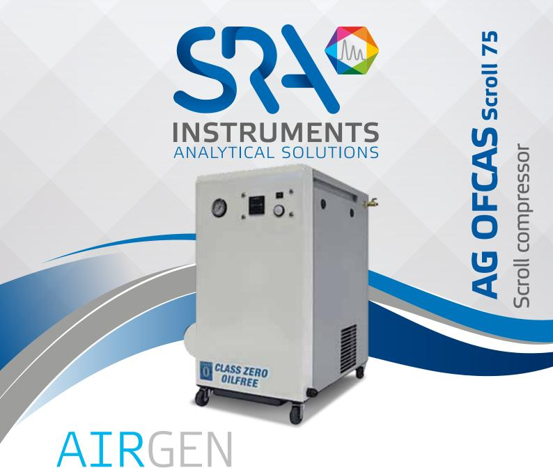
A scroll compressor uses two interleaving scrolls to compress air. Devices using this technology are known for operating more smoothly, quietly, and reliably than conventional compressors. Unlike pistons, the orbiting scroll's mass can be perfectly counterbalanced, with simple masses, to minimize vibrations. The scroll's gas processes are also more continuous. Additionally, a lack of dead space gives an increased volumetric efficiency.
