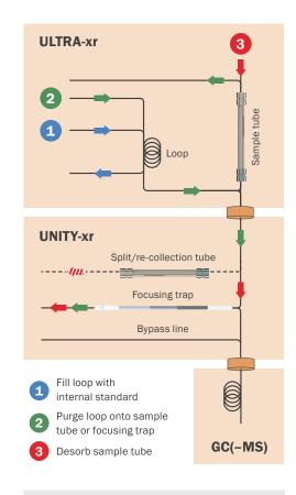
**For versatile method validation**, internal standards can be added to tubes or focusing traps on all ULTRA-xr systems.
