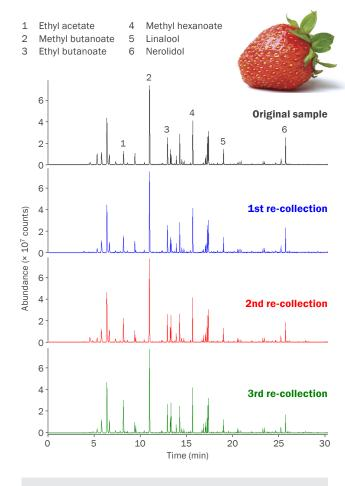
**Quantitative analysis** of the aroma profile of fresh strawberries is confirmed by three successive re-collections and repeat analyses of the same sample, each collected onto a clean sorbent tube.
