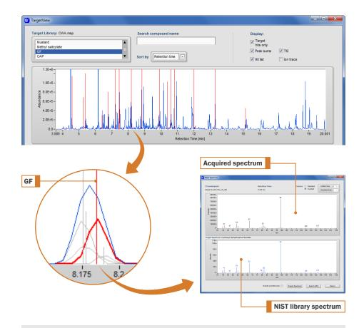
**Confident identification of 'GF' (cyclosarin)** in a sample of diesel oil is possible despite the complexity of the original chromatogram and the presence of co-eluting compounds (whose profiles are shown in grey in the inset).
