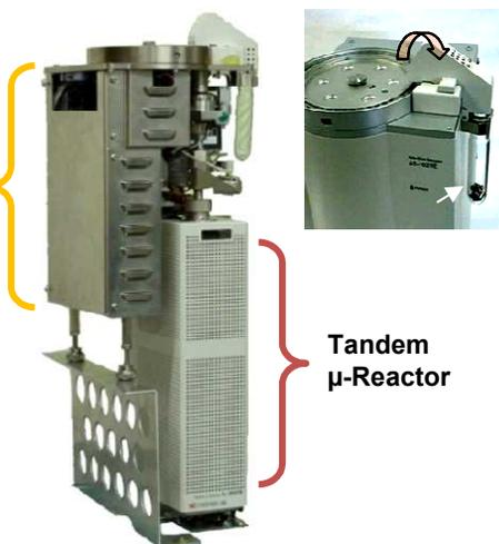
The analysis of solid samples can be automated using the Auto-Shot Sampler. The figure on the left (center) shows the Auto-Shot Sampler, with the housing cover removed, installed on the Tandem  $\mu$ -Reactor.
