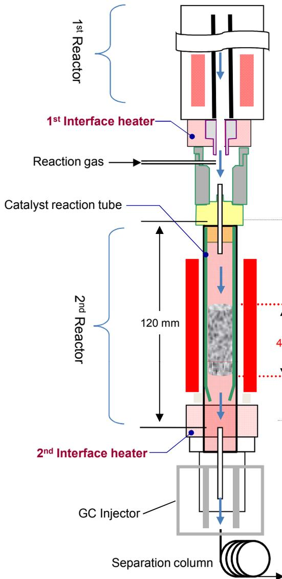
The thermal profile of the catalyst reaction tube inside the 2<sup>nd</sup> reactor between 100 and 900°C is shown in the figure below. The temperature variation within a 40 mm length of the catalyst bed is  $\pm 0.1^\circ\text{C}$  and the maximum temperature deviation is 3°C at 400°C. The reactor temperature can be easily calibrated using an external temperature sensor that is inserted into the center of the reactor.
