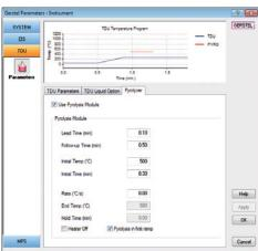
Thermal desorption prior to pyrolysis eliminates interfering contaminants, in this case C2 - C4 carboxylic acids
