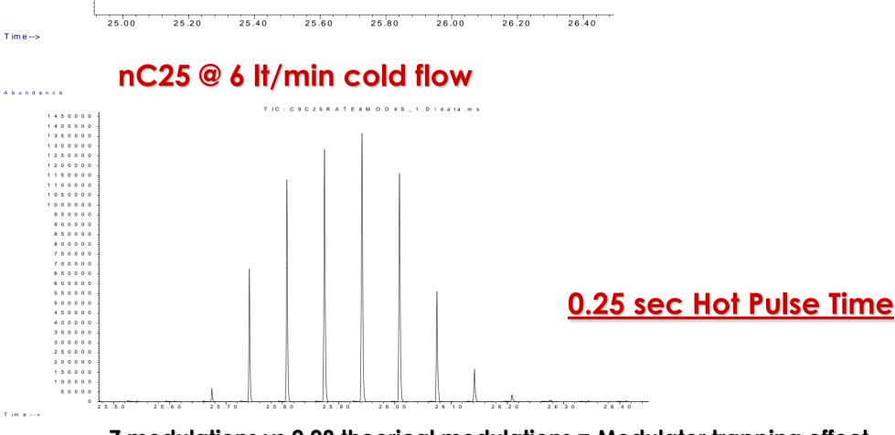
7 modulations vs 2.28 theorical modulations = Modulator trapping effect
