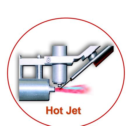
\*Hot Jet: flash heating to launch the trapped compounds
