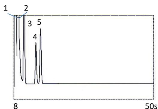
Natural gas analysis, with backflush at 8 seconds
