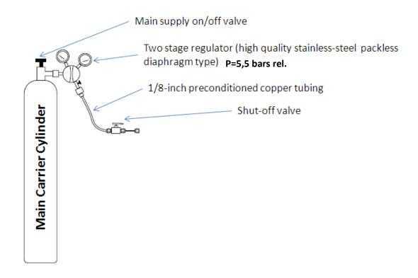
Set your input pressure between [530 and 570 kPa] [77 and 83 psi] [5.3 and 5.7 bars] Whenever the cylinder is changed, take care to purge the pessure reducer correctly to avoid contaminating the distribution circuit with air.
