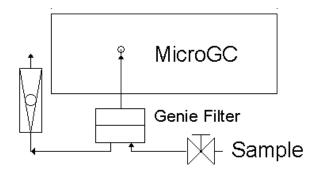
If there is a risk of condensation of the sample (organic solvents or high-boiling compounds), it is preferable to choose the same system installed in a heated and insulated box.
