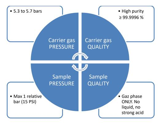
Not respecting these rules highly increases the risk of damaging your instrument. All standard procedures for using MicroGC are derived from these 4 golden rules: the quality of the carrier gas will require a tube purge to ensure this level of quality.
