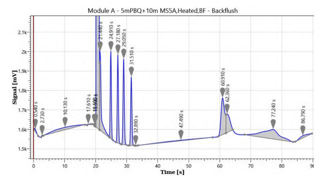
Considering the matrix peak does not require integration and no peak elutes in the backflush interference, we can exclude these regions from integration.
