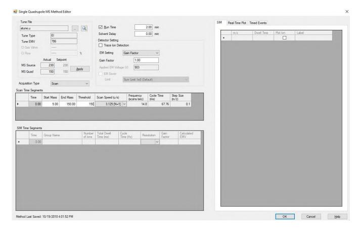
SRA recommends the above default settings, which should be modified according to the application. The Run Time must be equal to or greater than the Soprane CDS analysis time.
