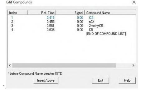
Right double-click on the chromatographic peak's apex to be added to define its retention time in the calibration. Define the name of the compound.
