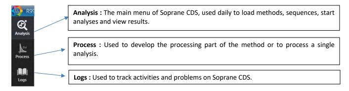
In each main menu, the most useful functions are accessible in the top bar:
