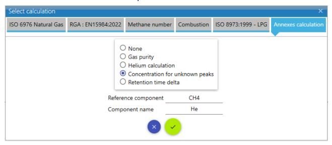
When this option is checked, a concentration estimate is calculated for the unknown components with reference to the calibration of a species identified and calibrated in the analytical method.
