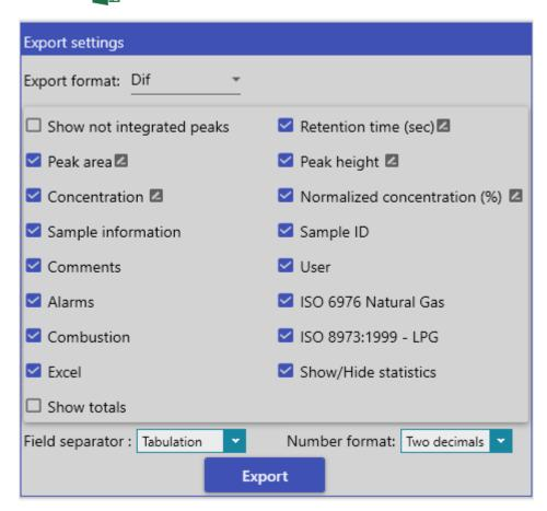
Soprane CDS enables to save the analysis results in files directly exploitable by a spreadsheet (DIF extension). These files are also visible in a text editor. The fields, whose value is in ASCII, are separated by a tab and the analyses by a line break.
