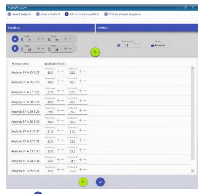
8. Click on to automatically create a sequence of analysis with one analysis for each method previously generated.
