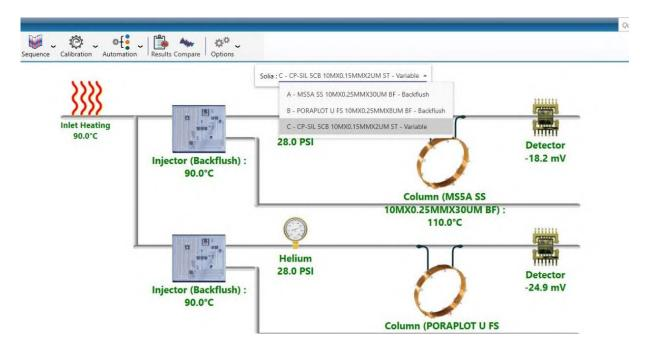
The names of the different modules are displayed on the screen. Click on the module to be coupled to the MS detector.
