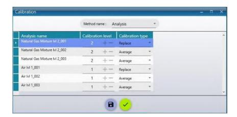
The  $N_2$  and  $CH_4$  peaks are reintegrated for the 3 natural gas analyses. The average area of the  $N_2$  and  $CH_4$  peaks is calculated. The average area of  $N_2$  peaks is associated with 1.6% and the mean surface area of  $CH_4$  peaks is associated with 94.43 % (level 2).
