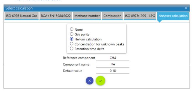
Helium estimation is related to ISO 6976 and natural gas analysis, it must be added to the ISO 6976 calculation option.
