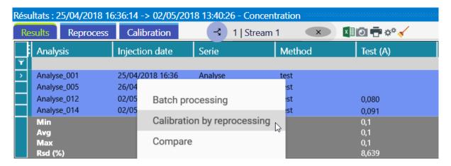
The first step consists in selecting the analyses to calibrate, then right-click on the analyses and click on Calibration by reprocessing (or with the menu Results > Calibration by reprocessing).
