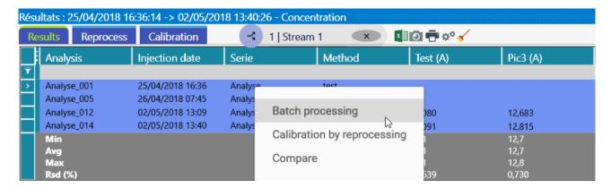
The first step consists in selecting the analyzes to be reprocessed, then right click on the analyzes and click on **Reprocessing** (or with the menu **Results> Reprocessing**).
