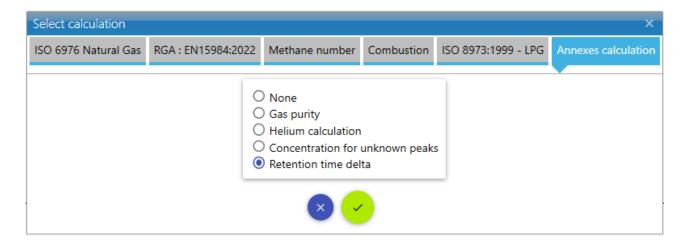
When this option is checked, the retention time delta is calculated between the expected retention time and the retention time.
