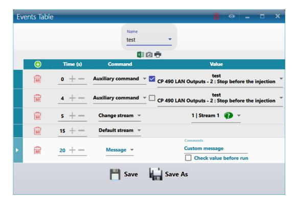
Soprane CDS will automatically start the analysis at the end of the events table.
