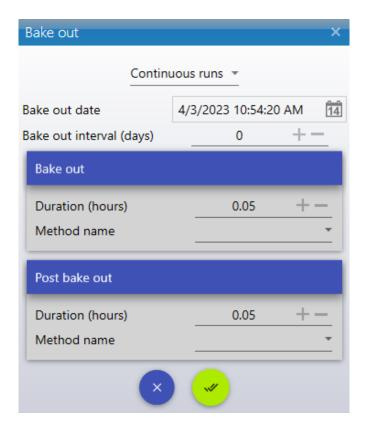
The bake out requires different parameters (higher column temperature, detector OFF) than those used for analysis, therefore you should indicate a bake out duration and the name of a method to be used for regeneration.
