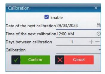
In order for the programming of a calibration to be detected, you must first **activate it by checking "Enable"**; if it is deactivated the calibration will not take place.
