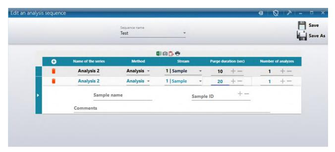
In this table, it is possible to define the analyses by giving them a name, to select an analysis method (each box is a list field displaying all the methods), to indicate which stream is concerned (another list field) and to specify the minimum sampling time before the injection and the number of repetitions of this step.
