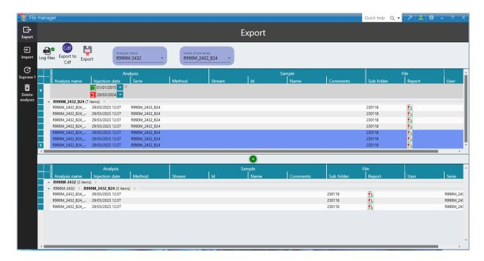
By default, the export mode is activated, the first data table contains all the analyses corresponding to the selected analyzer and series.
