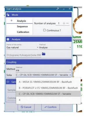
When writing an analysis sequence: the valve position will change between the analyses and during the sequence, in order to couple the desired  $\mu$ GC module to the MS detector for each analysis:
