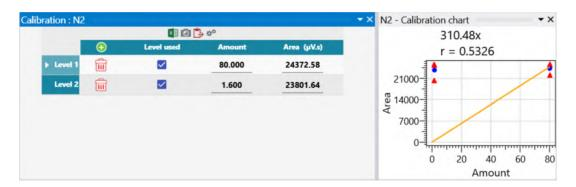
From this moment, if an analysis is started with the "Analysis" method, the chromatogram obtained will be automatically processed with the integration method and the identification table previously developed and the result in concentration will be linked to the calibration previously performed.
