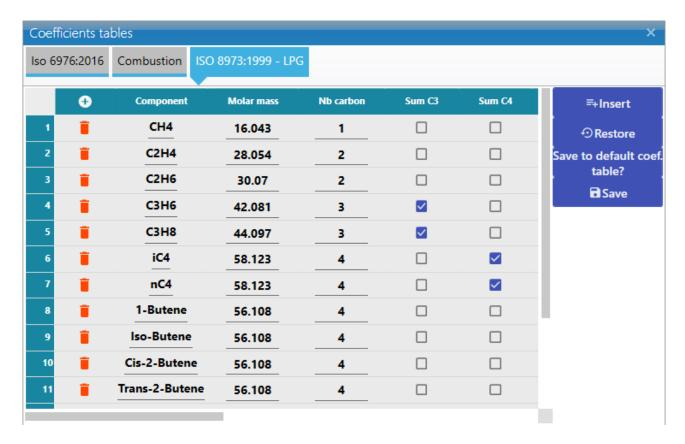
The table is composed of the columns "Component", "Molar mass", "Nb carbon", "Sum C3" "Sum C4", "Sum C5", and "Coef. M Vol", "Abs. press. vapor @ 37.8, @ 40, @ 50 and @ 70°C", "Olefines" and "Index fact. Octane".
