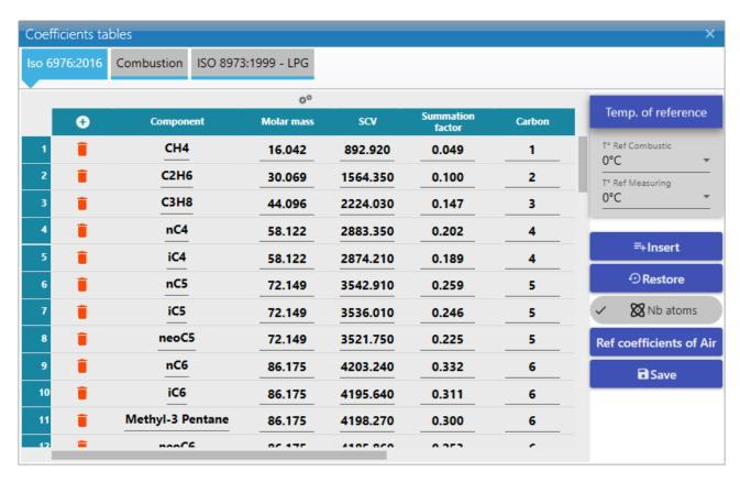
The table is composed of the columns "Component", "Molecular mass", "SCV" and "Summation factor". For each reference compound you will find its molar mass, reference SCV as a function of reference temperature conditions as well as the summation factor which also varies according to the reference conditions.
