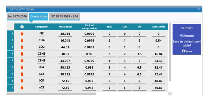
The table is composed of the columns "Component", "Molar mass", "Fact. of compression", "H2O", "CO2", "O2", "Coef. comb.", "Critical temp.", "Critical press.", "Coef. 2 degree", "Coef. 1 degree", "Constant".
