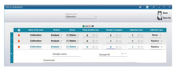
In this table, it is possible to **define the analyses by giving them a name**, to **select an analysis method** (each box is a list field displaying all the methods), to indicate **which stream is concerned** (another list field) and to specify the **minimum sampling time before the injection** and the **number of repetitions of this step**.
