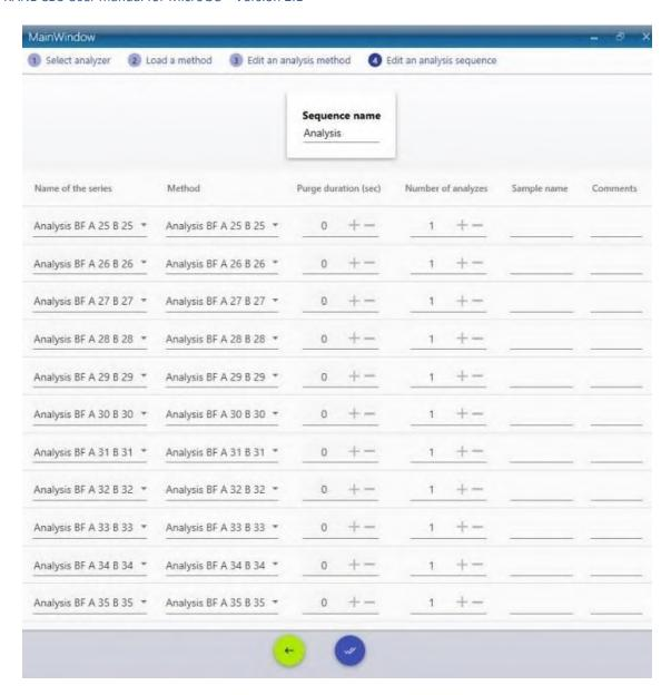
10. Connect a standard containing CH<sub>4</sub> to the MicroGC, open Soprane CDS, click on "Start" and launch the previously generated sequence (see chapter Starting a sequence):
