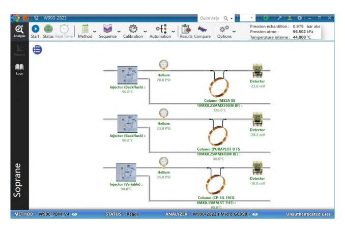
If an element has not reached its set point, it means that it is not ready. The text is in Orange.
