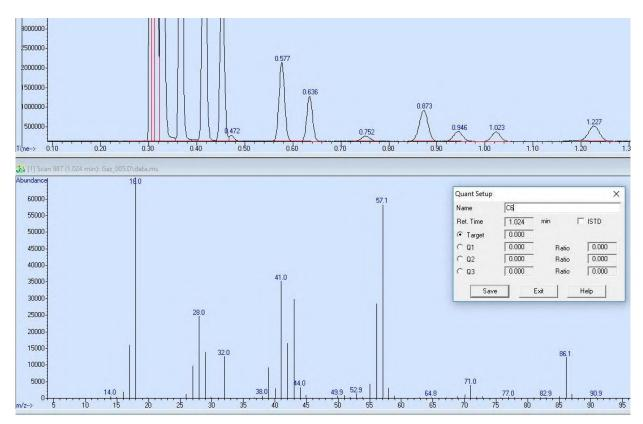
At this stage, it is also possible to select target ions used for quantification. To do this, click simultaneously on the left click and right click on the m/z peak of the mass spectrum to be considered.
