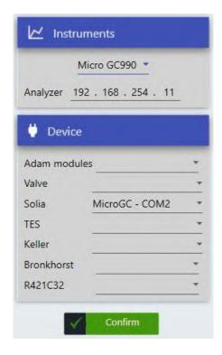
From Soprane Configurator, create a new analyzer by clicking on the "+" icon. Then enter the IP address of the instrument. Select "COM2" for the Solia category (as shown in the image above).
