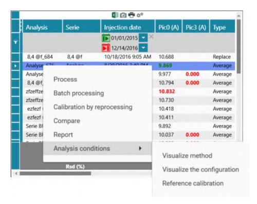
The second way is from the **Process** tab. Select the "Calibration" menu and click on "Reference Calibration".
