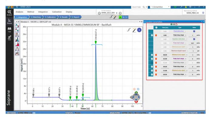
The "Integration Parameters" are used to define how to integrate the peaks on the chromatogram. In the "Integration Parameters" table, a row corresponds to an integration parameter. For each line, it is necessary to define the "Time" from which the parameter must be applied until the end of the chromatogram or the definition of another similar parameter, the "Type" of integration parameter to be applied and its "Value".
