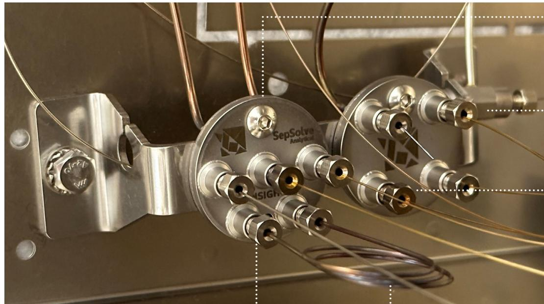
**Innovative design** to ensure the widest possible volatility range ( $C_1$  to  $C_{60}$ ), and the flexibility to perform heart-cutting, splitting for parallel detection or backflushing.
