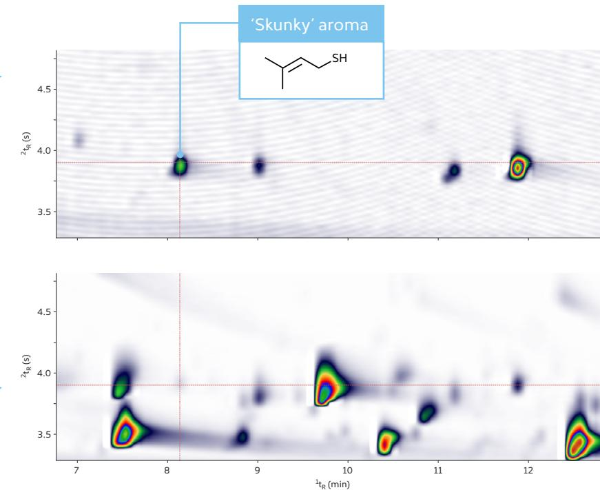
In this analysis of beer aroma, profiling benefits from confident identification by mass spectrometry (MS) and precise quantitation of sulfur species by sulfur chemiluminescence detection (SCD).
