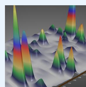
Enhanced separation by GC $\times$ GC using INSIGHT® modulation for full sample characterisation.
