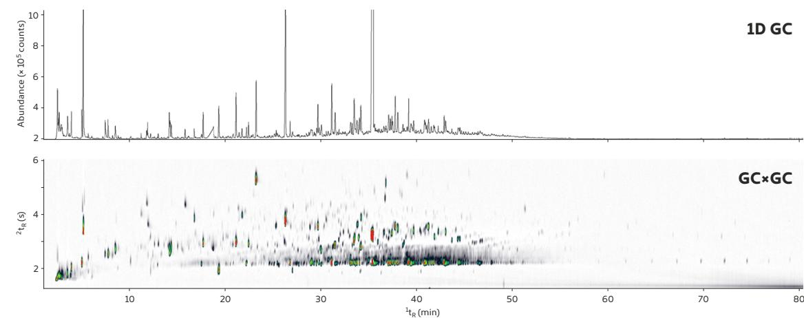
For this complex sample, GCxGC resolves about 10 times as many compounds as 1D GC – typical of the improvement in separating power that a well-chosen modulator can provide.
