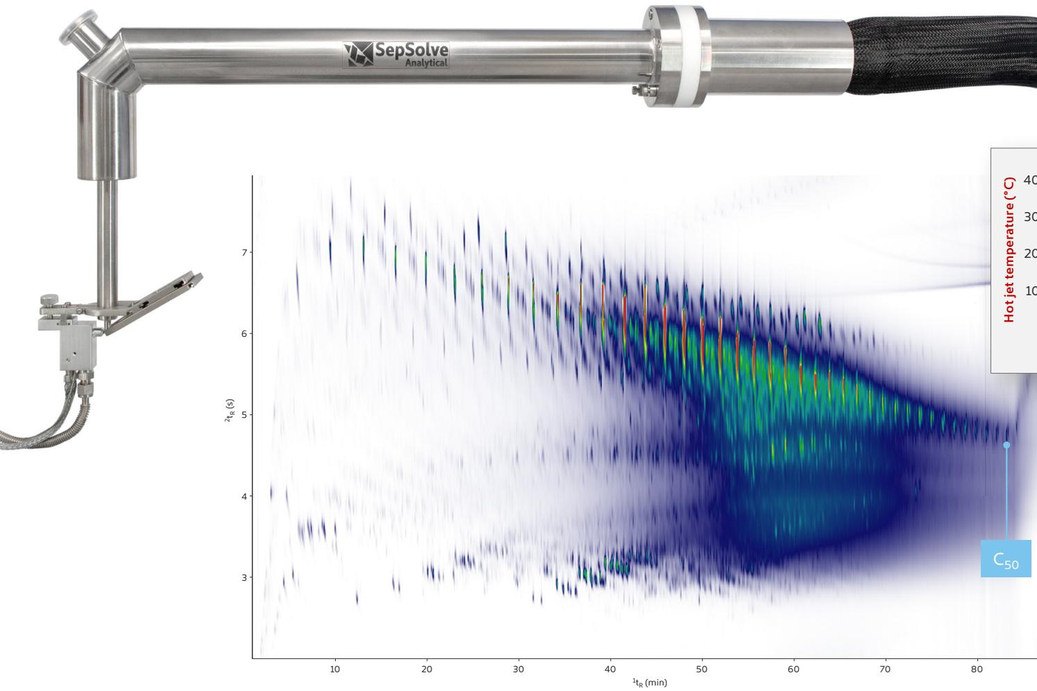
In this vacuum gas oil, over 3000 peaks were resolved using GCxGC-FID with INSIGHT-Thermal, with advanced jet control (including the ramped flow rates, shown inset) providing efficient modulation of high-boilers.
