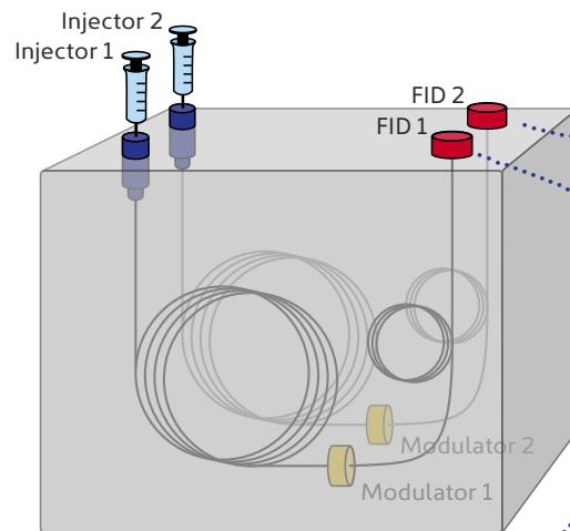
Using two INSIGHT-Flow modulators in a dual-channel configuration immediately doubles productivity, for a swift return on investment. This is illustrated for environmental monitoring of total petroleum hydrocarbons (TPH), with full instrument control and group-type data analysis in SepSolve's ChromSpace® software.
