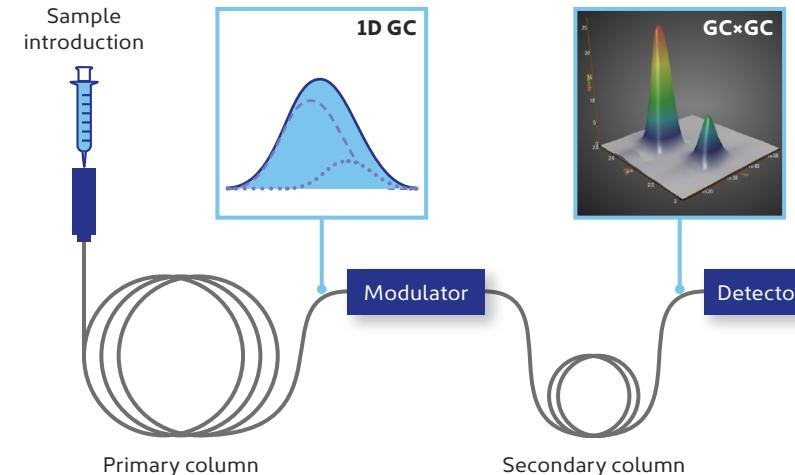
A typical analytical system for GCxGC, showing how the modulator has a central role in coupling the primary and secondary columns, and so enabling the separation of two peaks that have overlapped in 1D GC.
