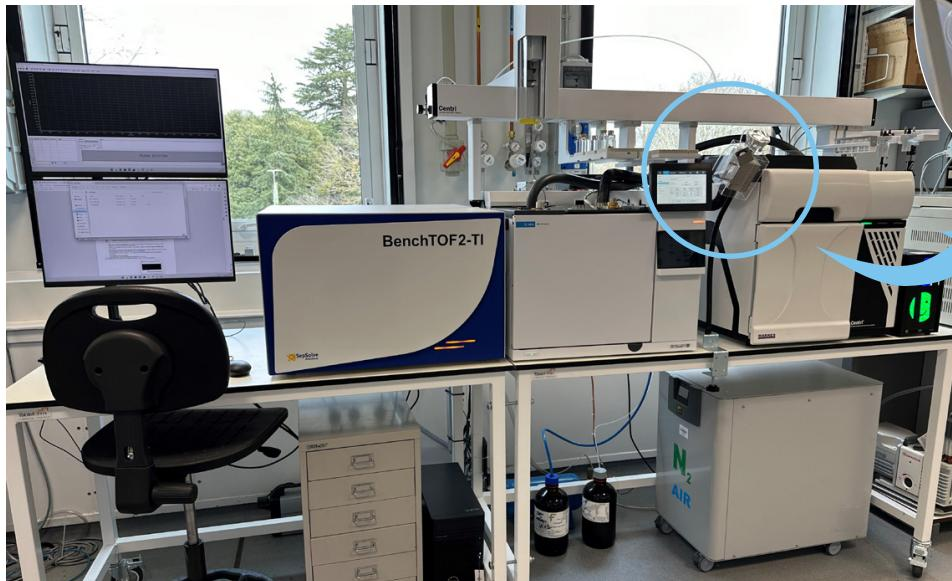
A custom-built SepSolve system at the University of Reading (UK) for advanced analytical and sensory characterisation of food. The setup comprises Markes International's Centri® extraction and enrichment platform, SepSolve's own INSIGHT-Flow GC $\times$ GC and BenchTOF2™ time-of-flight mass spectrometer, and an olfactometry port from GL Sciences.
