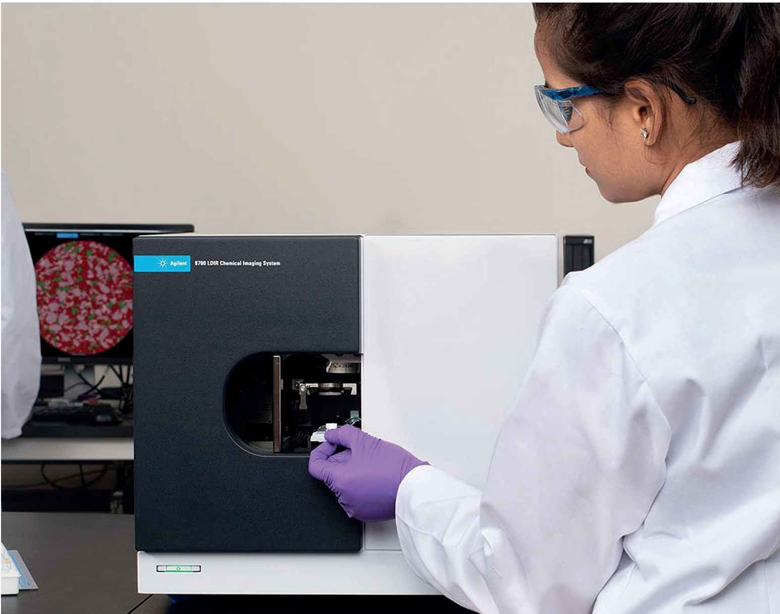
Agilent 8700 Laser Direct Infrared Imaging system for fast and automated analysis of microplastics in environmental samples.
