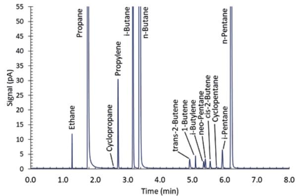
The LGI method for determining oily residue in C3 and C4 streams complies with ASTM D7756 and EN 16423. Adding an external oven with a liquid sample valve configuration to a high pressure liquid sampling application allows a simultaneous analysis of the oily residue (ASTM D7756/EN 16423) and the hydrocarbon composition (ASTM D2163 & ISO 7941) of LPG from the same sample cylinder.
