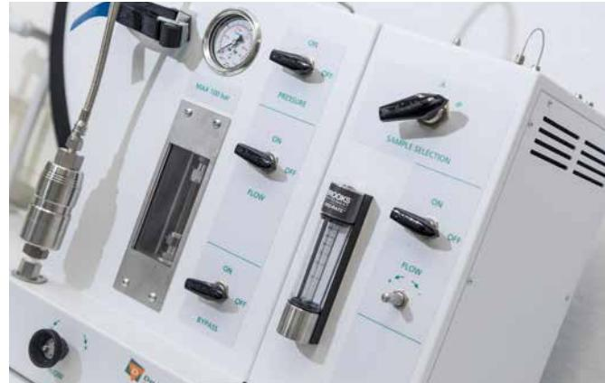
For a repeatable introduction into a GC system the liquefied gas sample must remain in a liquid phase under constant pressure during the GC injection. This is especially required for LPG or other liquefied gases.
