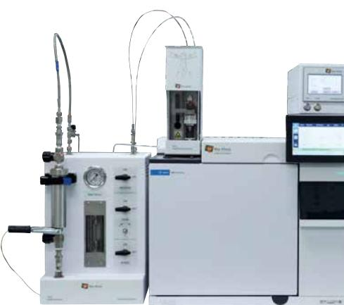
To quantify Amines in LPG an LGI system is configured according to ASTM D7756. The application uses a Nitrogen Phosphorus Detector (NPD) for a selective nitrogen detection. In a single run both the oily residue and desulfurization agents such as Diisopropanol Amine (DIPA) and Dibutyl Amine (DBA) are determined.
