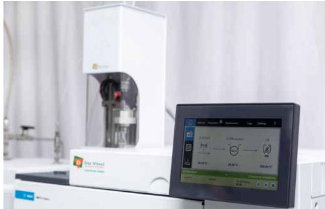
**The direct injection approach of the Liquefied Gas Injector (LGI) is a safe alternative technique to a liquid sampling valve or manual evaporation.**
