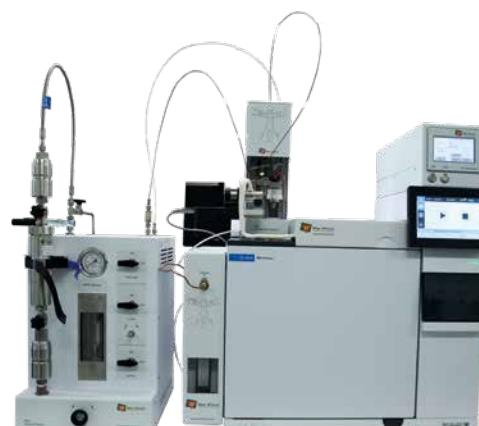
The application can also be used as an alternative to ASTM D1157 to determine TBC inhibitor or to ASTM D1025 for the analysis of Residue (C10 - C24 oily residue).
