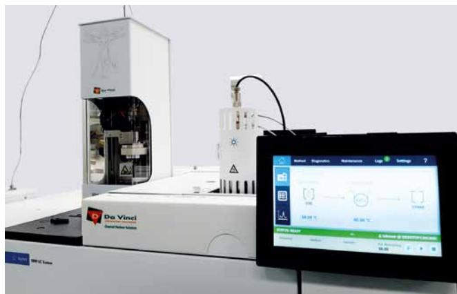
The elemental Sulfur GC application is based on the ASTM D7756 configuration including the DVLS Pressure Station and Liquefied Gas Injector to safely handle and inject LPG samples. The direct injection technique of the LGI ensures full transfer of the elemental sulfur component onto the column.
