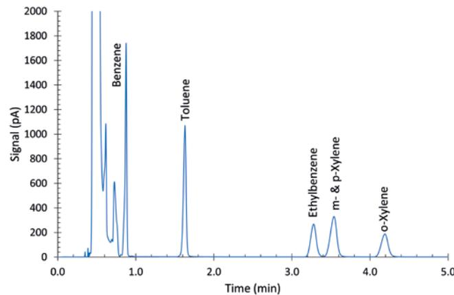
The Benzene & Toluene analysis is described in ASTM method D7756 Appendix X3 and includes the Liquefied Gas Injector and Pressure Station. In a single run the application determines both the Benzene, Toluene and oily residue in LPG.
